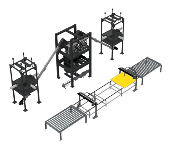
Our machine consist of two silo's or bigbag stations, for storage of concrete pre-mix, two high power double shift mixer units for mixing the concrete, a concrete pump and an linear axis application tool that shoots the material in moulds that are transported with a conveyor belt.
